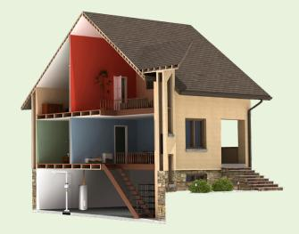
The BC Building Code requirements for radon vary by year and region. Some homes have a radon stub pipe or an extended pipe that runs through the house. These features are the beginning of a radon mitigation system and can make installation easier. Long-term (91 day) testing is still necessary.
